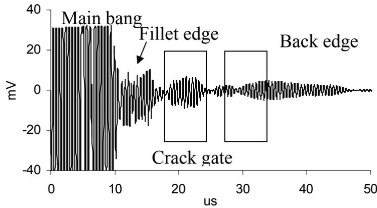
Figure 4. Example software gates for analysis of data.
