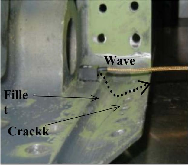
Figure 5. Transducer position and wave propagation direction.
