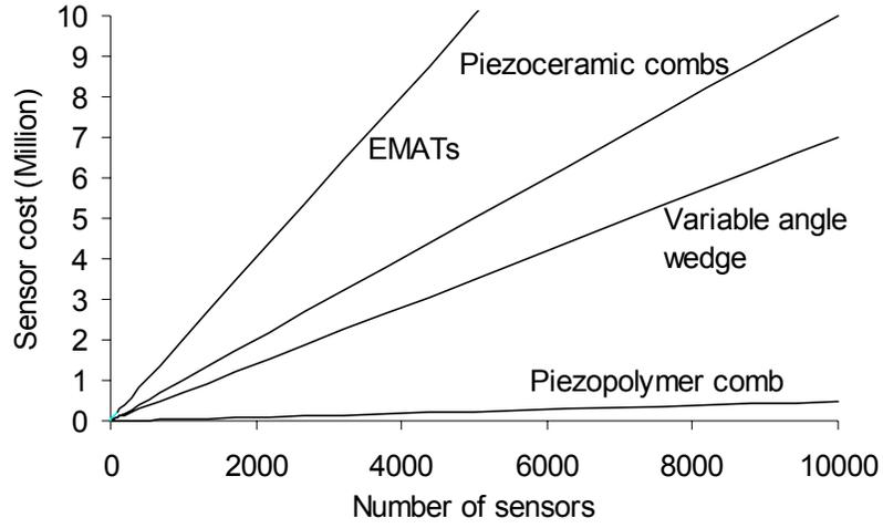
Figure 3. High volume application of guided wave sensors
