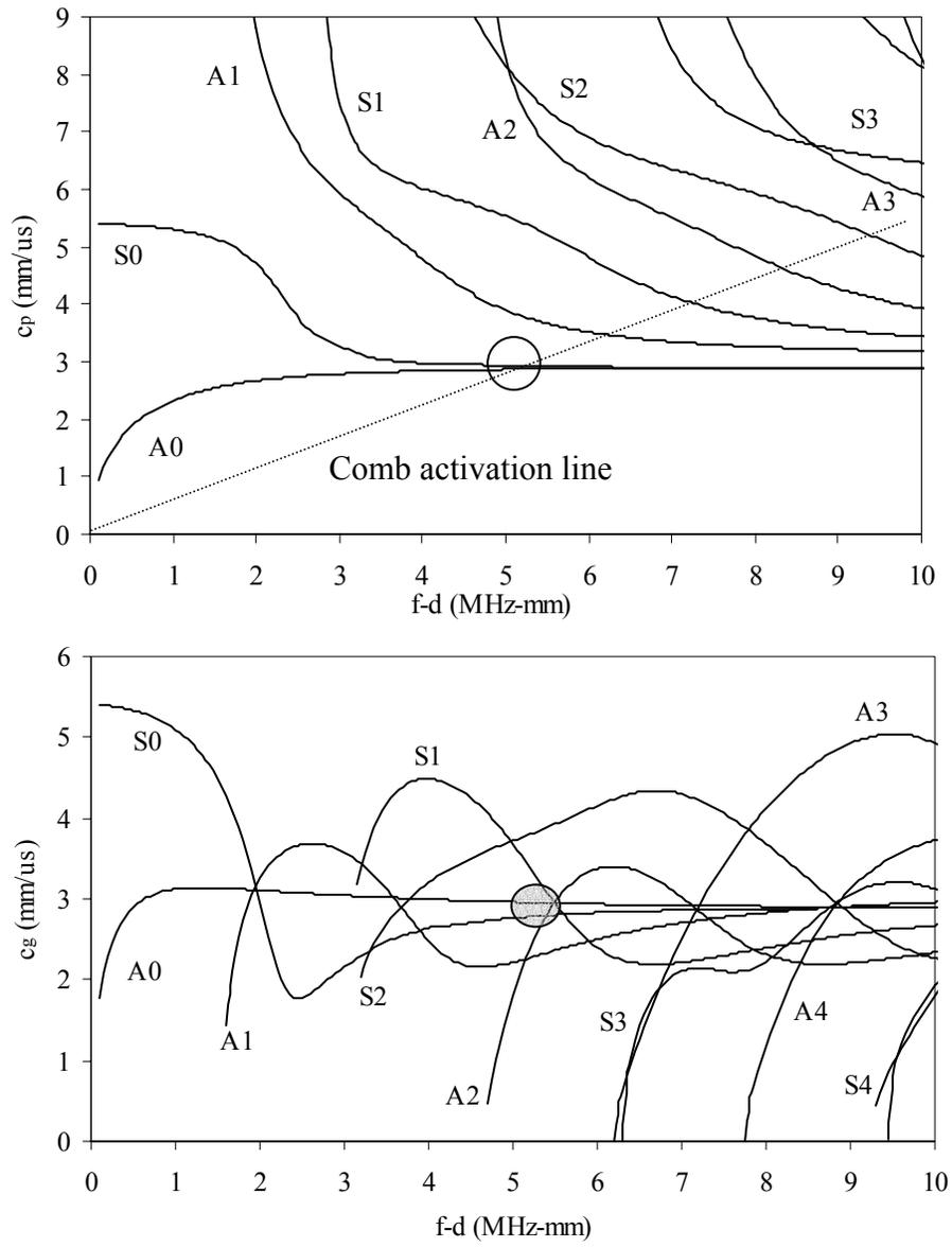
Figure 7. Phase (top) and group (bottom) velocity curves for an aluminum plate.
