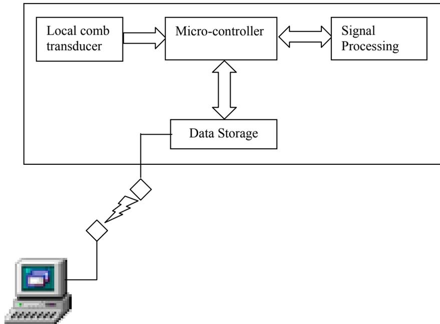
Figure 8. Wireless communication with guided wave sensor.
